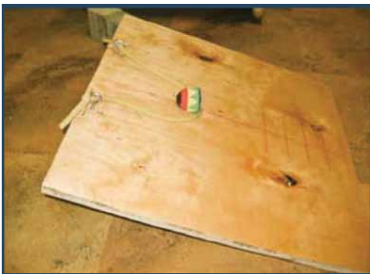
An example of a projectile system created and optimized for this class. The factors that were varied include board angle, elastic pull back position, ball position and peg location.
