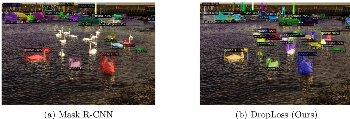
Figure 3.5: Qualitative results of a Mask R-CNN baseline and b the proposed DropLoss. Instances with score > 0.5 are shown. DropLoss adaptively removes background proposal losses of rare and common categories to reduce bias towards misclassifying these objects as background. In this case, the common category ‘goose’ is misclassified as background in a , and correctly identified in b .
