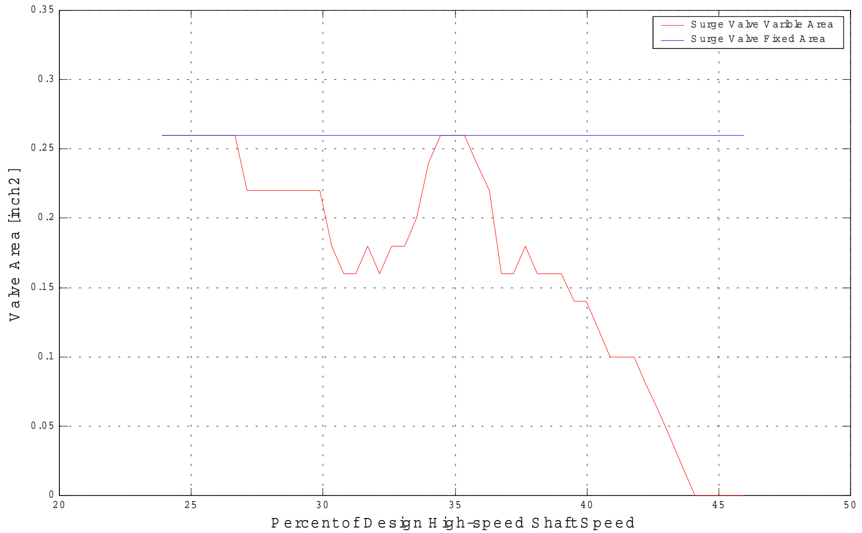
Figure 6-10. Variable valve area schedule comparison to fixed valve area.
