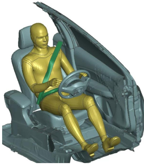
Figure 6-1 GHBMC model seated in driver position
