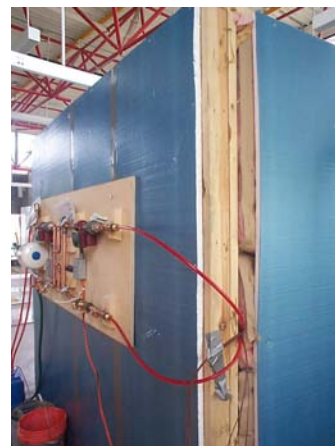
Figure 4-3-1-4b: Hot Water Circulation Loop (inlet-outlet side view)
