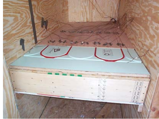
Figure 4-3-2-7b: Warmboard 12" o.c Construction (2)
