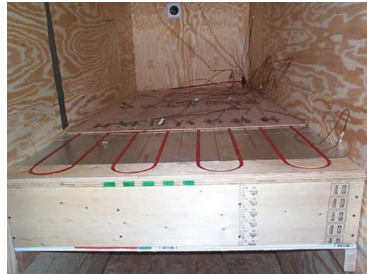
Figure 4-3-2-1b: RAUPANEL 6" o.c Construction (2)
