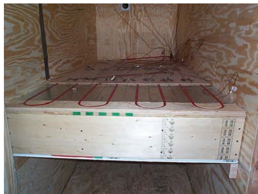
Figure 4-3-2-2b: RAUPANEL 6" o.c w/o insulation Construction (2)
