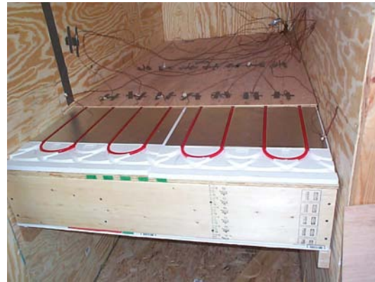
Figure 4-3-2-8b: Roth 6" o.c Construction (2)
