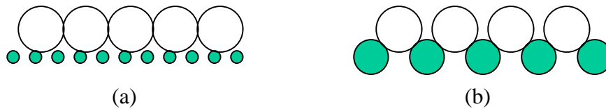
Figure 1.7. Postulated interaction between the cake particulates and the filter media (Willis, 1986).
