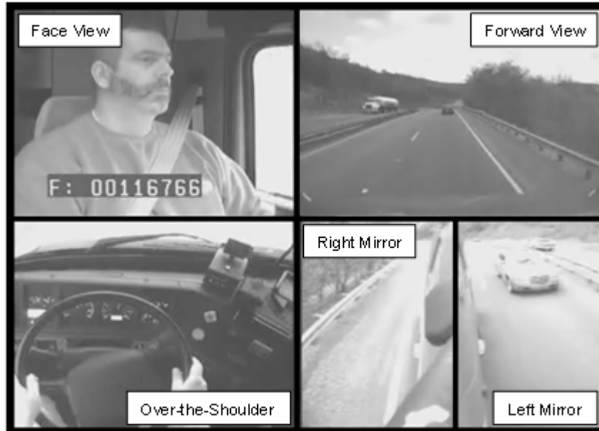
Figure 1. Photo. Five camera images multiplexed into a single image (driver is a VTTI employee and not a study participant).
