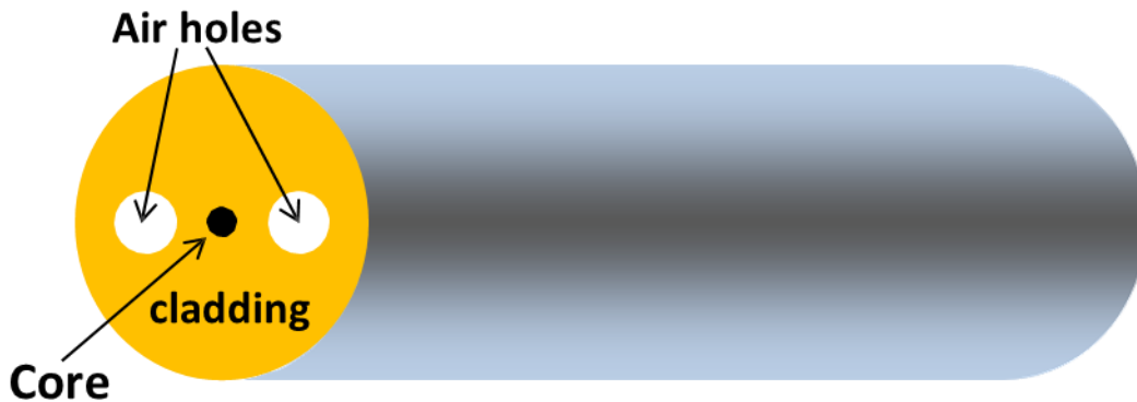
Figure 2.1 structure of side-hole fiber
