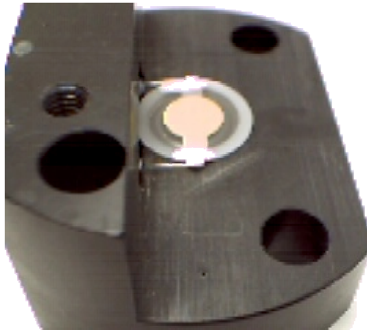
Figure 15. Base of the cell used to mount the crystal for experiments with a crystal in place. The gold crystal rests on an o-ring whose diameter is larger than the diameter of the central gold electrode. Spring clamps (wires on either side of the crystal) are bound to the electrode tabs using conducting silver paint to increase the stability.
