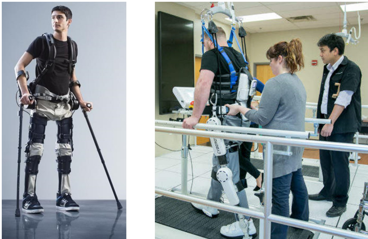
Figure 1: SuitX's Phoenix (left) [5] and Cyberdyne's HAL (right) [6]. Both exoskeletons require walking aids to balance.
