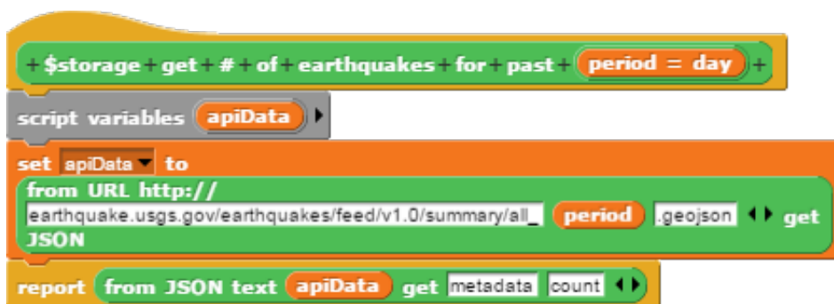
Figure B.5: The “get number of earthquakes for past (period)” block definition.
