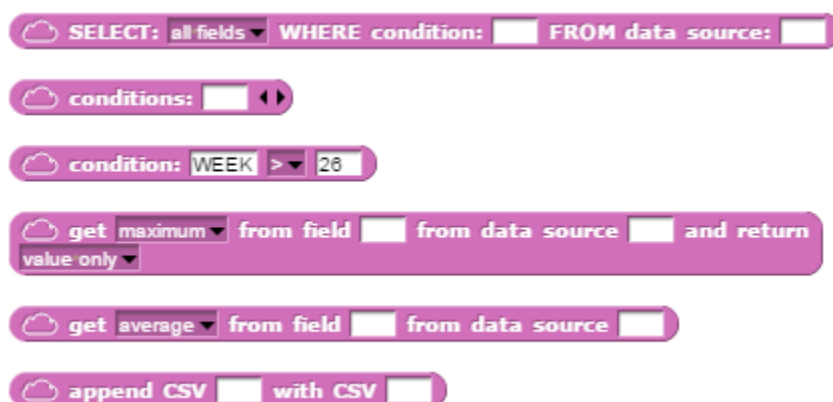
Figure 3.11: The big data processing blocks within the internal data process module in DataSnap
