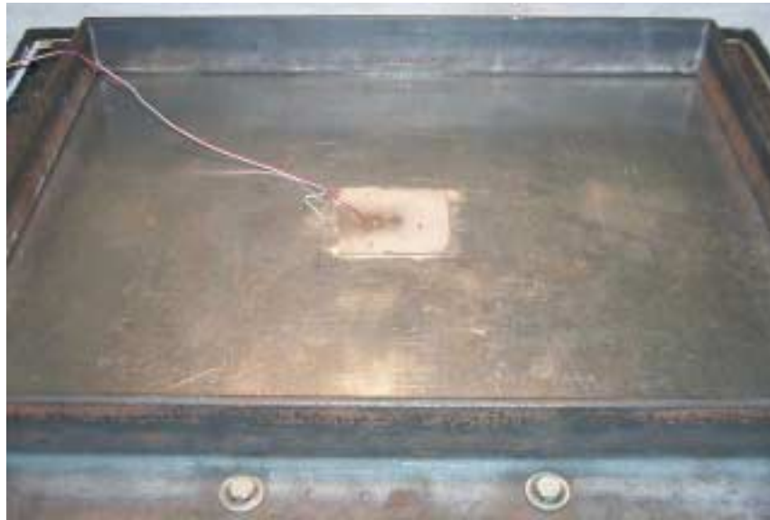
Figure 4.4. PZT Bonded to the Surface of the Test Plate.
