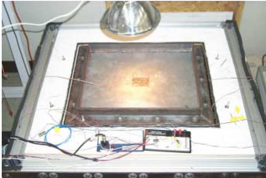
Figure 4.6. Overall Setup with Heat Lamp and Signal Conditioning Circuits.
