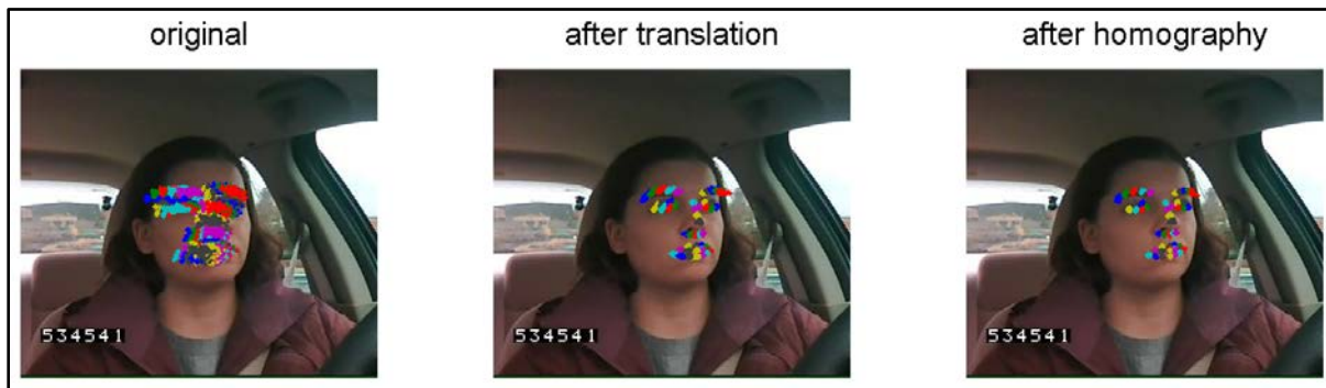
Figure 11. Screenshots. Frame registration showing improvement in consecutive frames. The original scatter sequence shows how fiducial points move with time. After homography, the movement of fiducial points has been minimized.
