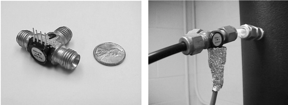
Figure 3.5 Sensym pressure transducer mounted in a T-connection
