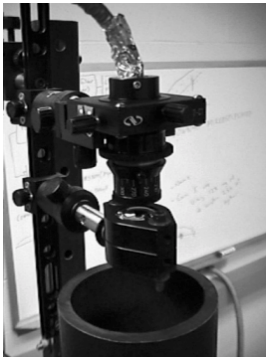
Figure 3.8 Lenses and fiber optics setup on top of the tube combustor
