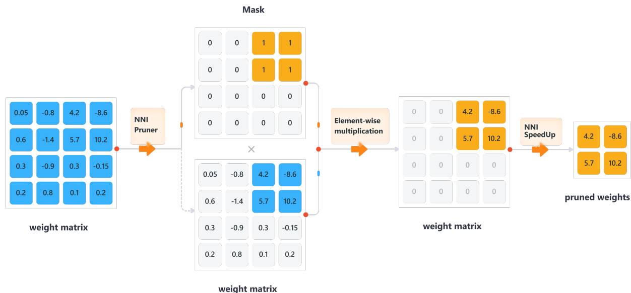
Figure 4.3: Overview of Pruning and Model Speedup using NNI Toolkit.
