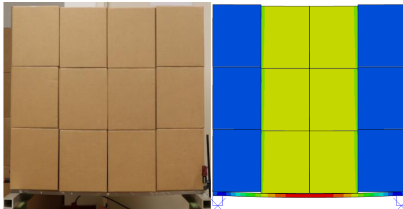
(c) 4 Columns – 3 Layers Unit Load
