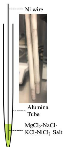
Figure 2-2 Ni/NiCl 2 thermodynamic reference electrode setup
