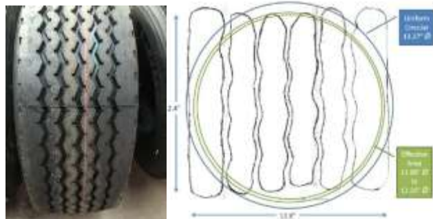
Figure 2-5 425 /65R22.5 Tire and contact imprint (Gibson et al., 2012)
