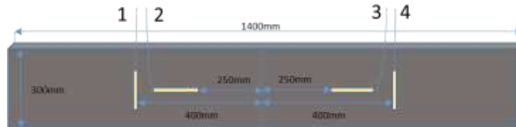
Figure 2-3 Strain gauge instrumentation schematic at underside of test slab
