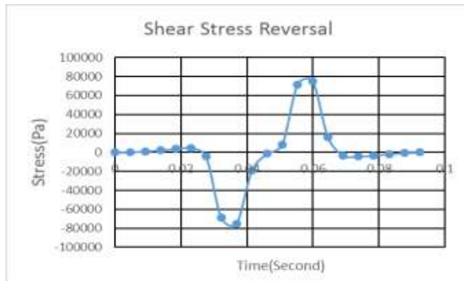
Figure 4-15 Shear stress reversal vs. time
