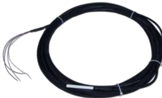
Figure 3-4 Temperature probe (107 temperature sensor, 2016)
