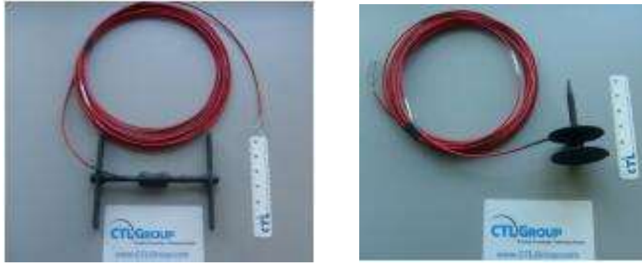
Figure 3-1 Asphalt mixture Strain gauges (Timm et al. 2004)
