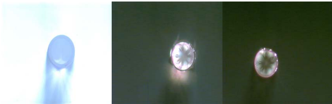
(b) After being exposed to 13.3% HF for 20min, 30min and to 18.6% HF for 10 min the fiber is around 52 \mu\text{m} , 49 \mu\text{m} and 45 \mu\text{m} in diameter(50 times magnification of the cutoff of the fiber tip).
