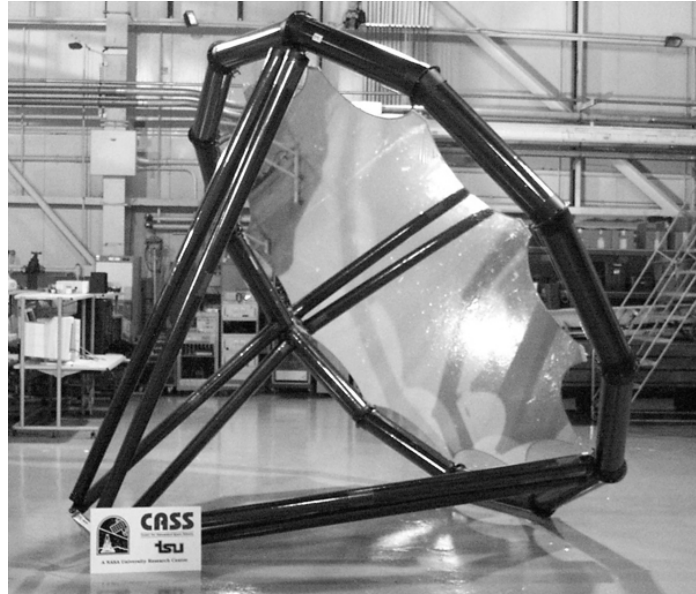
Figure 2.4: The inflatable hexapod structure for dynamic analysis. Photo courtesy of NASA / L. Horta.
