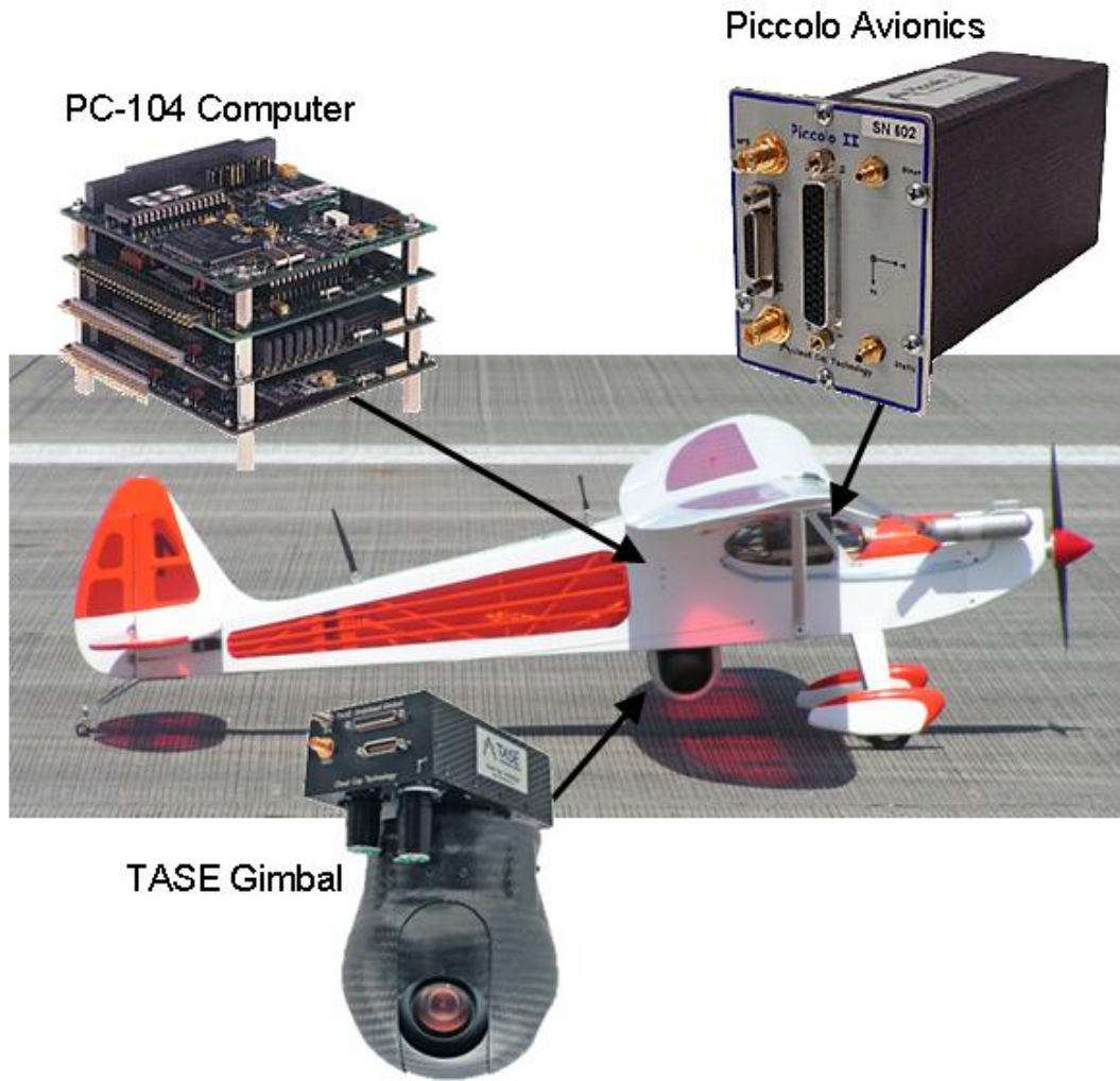
Figure 2.2: The VT Rascal with major components highlighted
