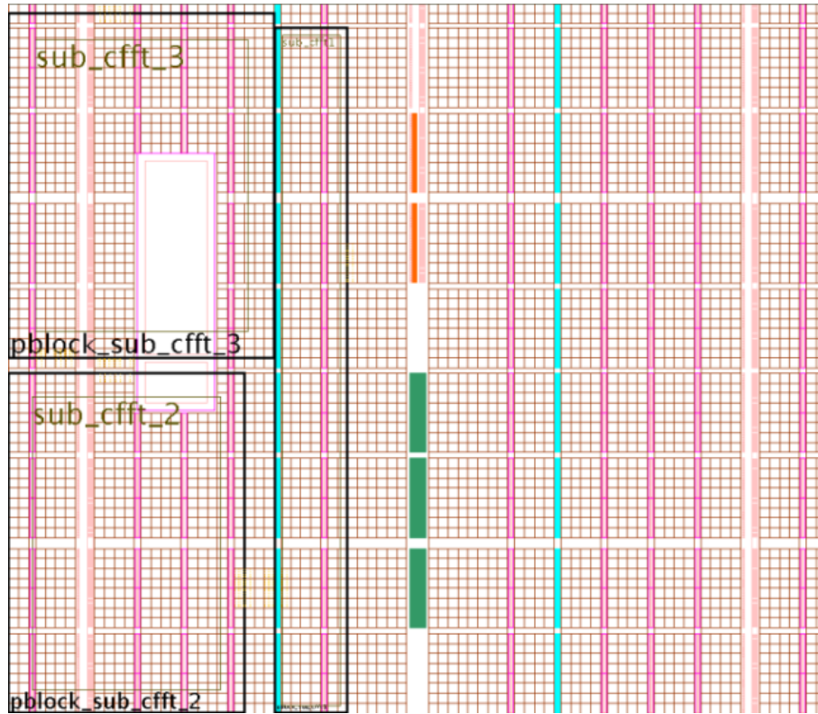
Figure 4.11: Sample floorplan (Screenshot captured from PlanAhead tool)
