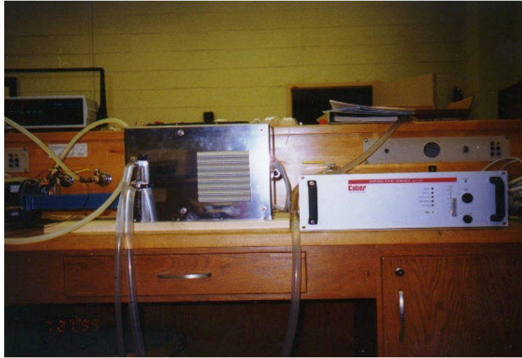
Figure 3.3: Picture of microwave power generator and remote launcher
