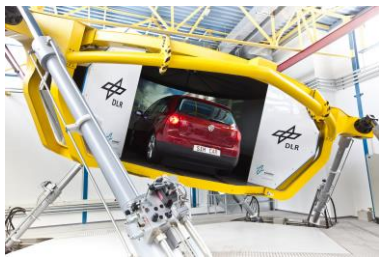
Fig.2: Dynamic driving simulator at the German Aerospace Centre (DLR). Photo from DLR Braunschweig.
