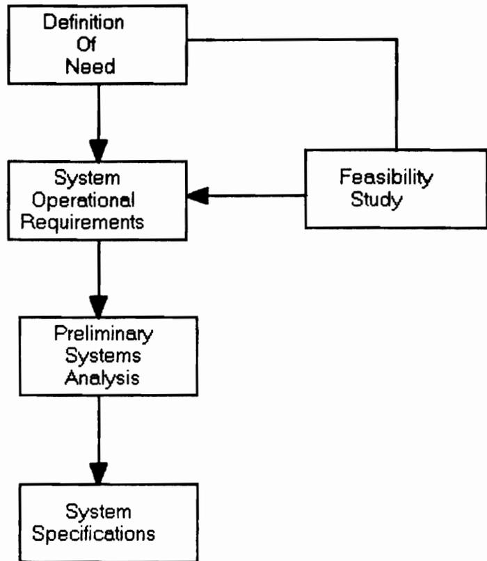
Figure. 2.1 Conceptual Design Flow
