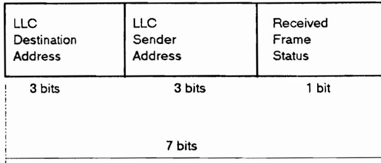
Figure 7.4 Acknowledgment Frame
