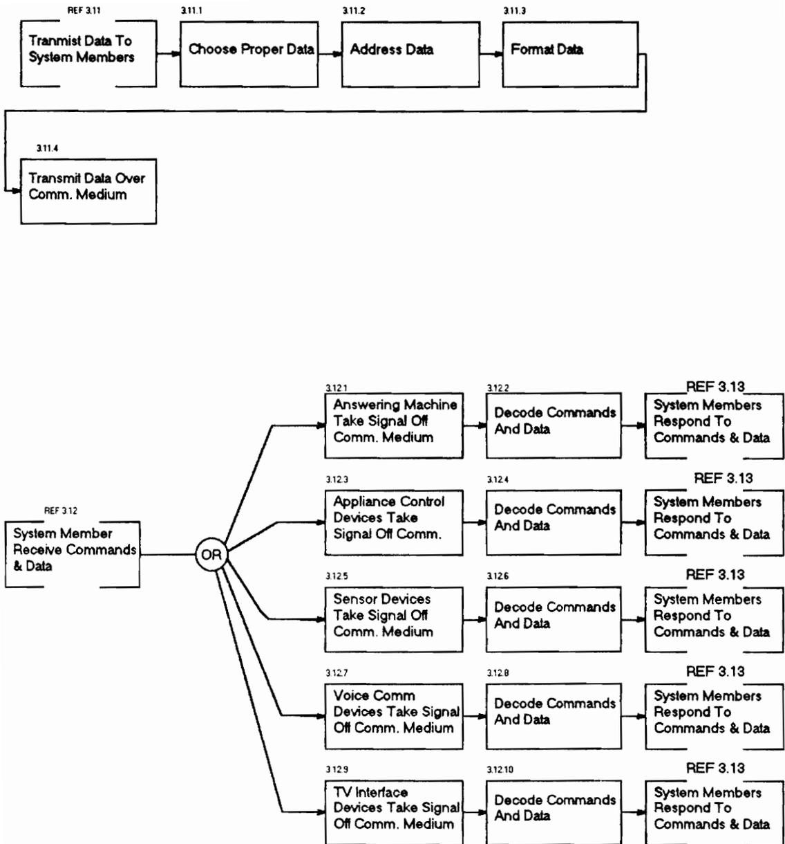
Figure 6.1 Home Automation System Functional Flow Diagram Cont.
