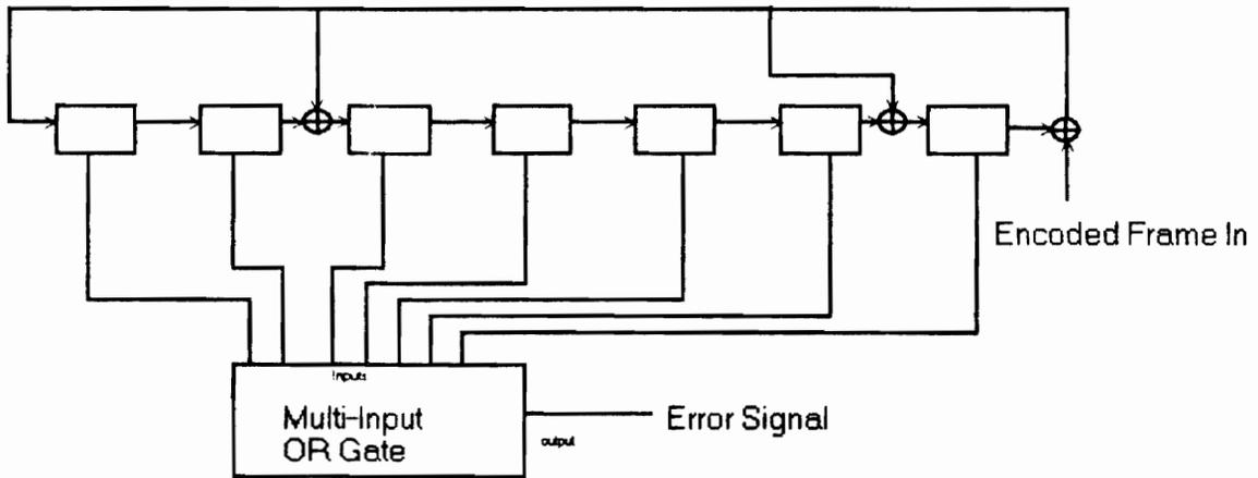
Figure 7.10 Home Automation System Error Detection Decoder
