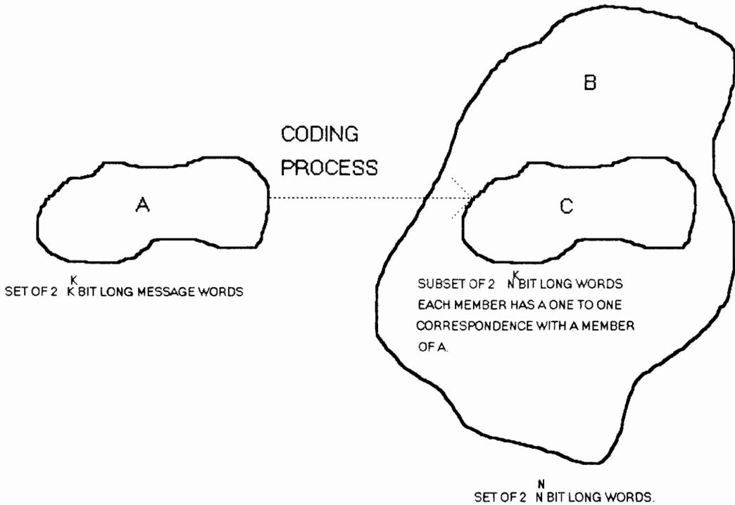
Figure 7.8 Example Of Coding
