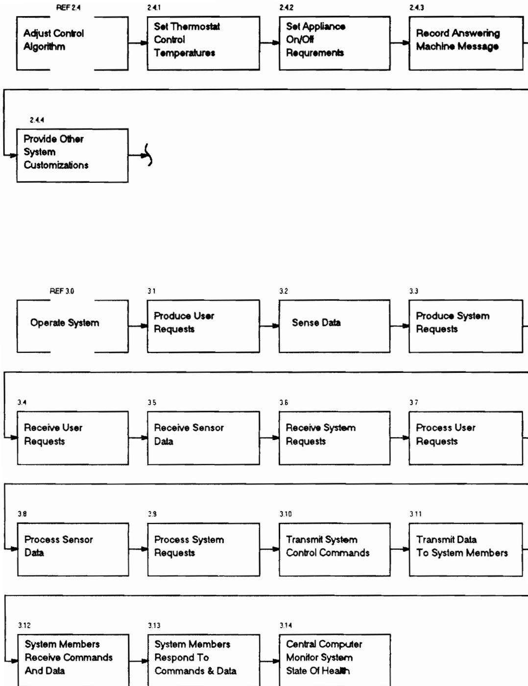
Figure 6.1 Home Automation System Functional Flow Diagram Cont.
