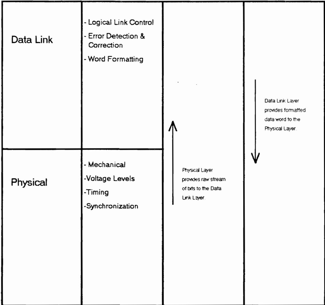
**Figure 7.1 Home Automation System Utilization Of OSI Layers**
