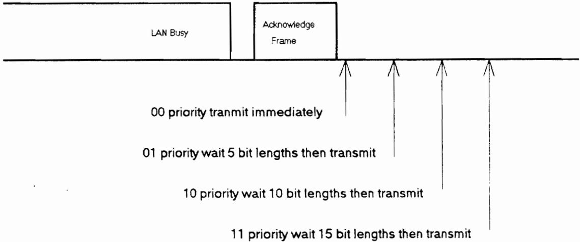
Figure 7.6 Retransmission Algorithm
