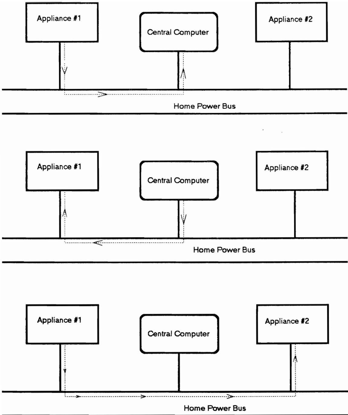
Figure 7.7 home automation system LAN Signal Types
