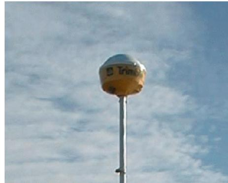
**Figure 3.** Trimble Combination GPS and OmniSTAR antenna.
