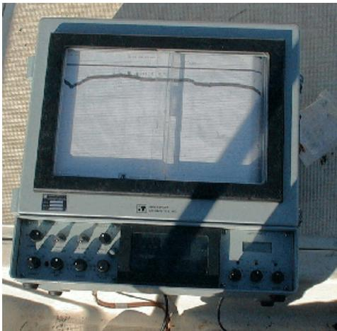
**Figure 4.** ITI Model 448 Ultrasonic Depth Sounder.
