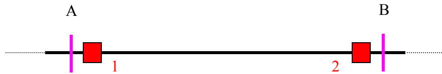
Figure 3-2 Transmission Line and Circuit Breakers
