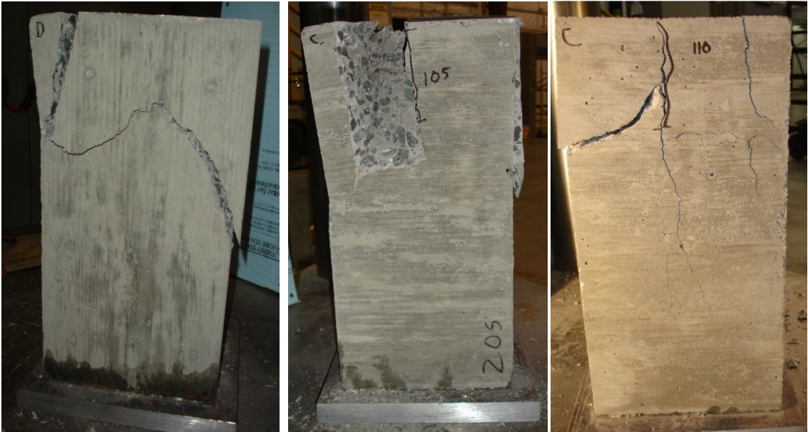
Figure 4-10: Failed Prisms with Spiral Reinforced
