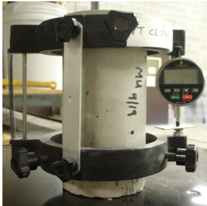
Figure 3-8: External Strain Gage for a 4 in. x 8 in. cylinder
