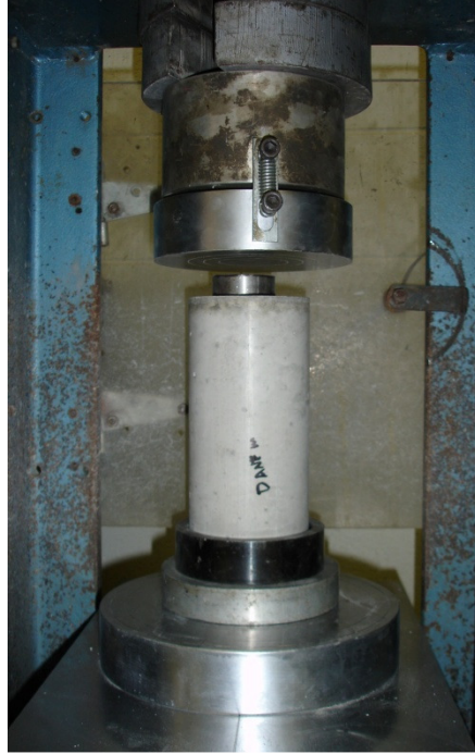
Figure 3-9: Cylinder Test Setup
