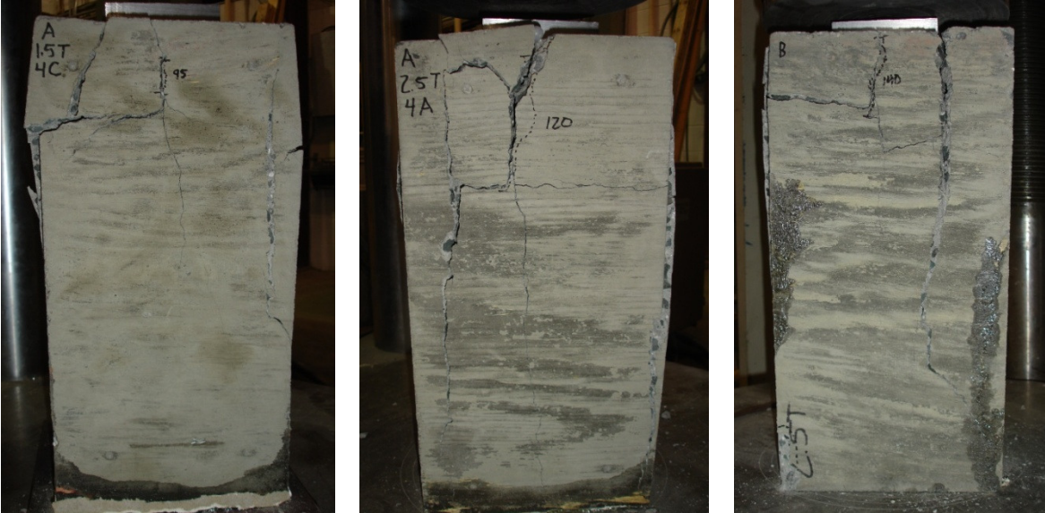
Figure 4-9: Failed Prisms with Tied Reinforcing
