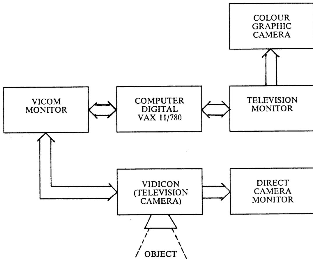
Figure 9. Digital Image Processing System (GIPSY).
