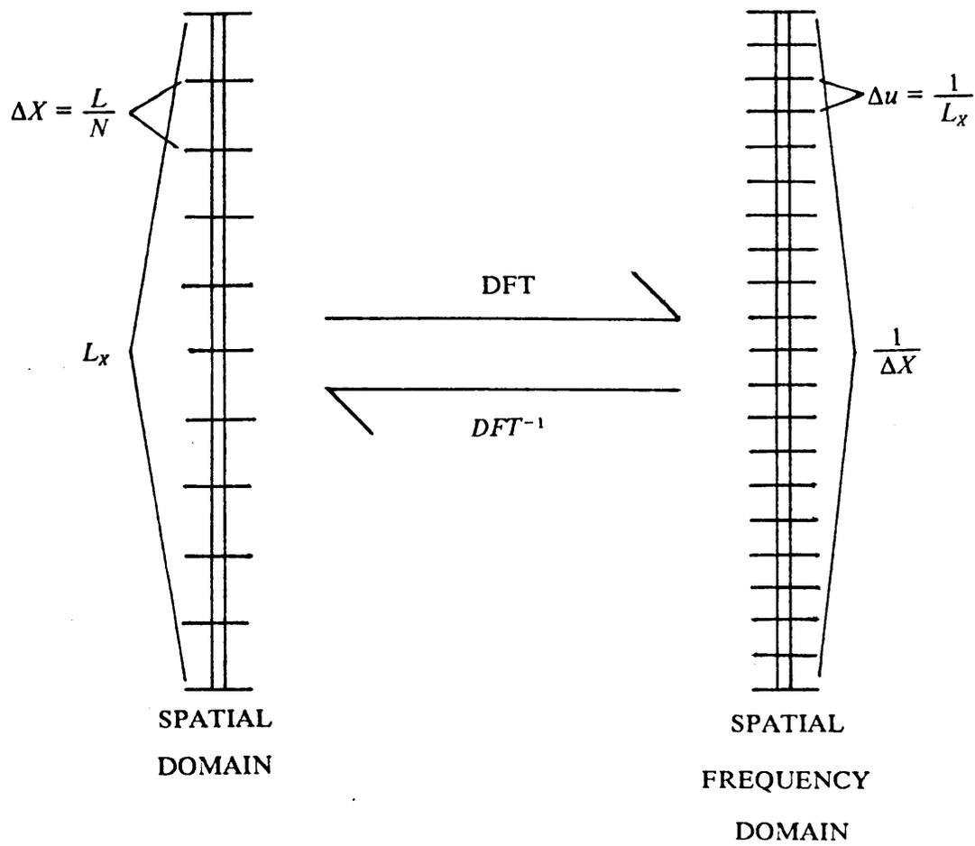
Figure 10. Geometric interpretation of 1-D transform parameter.
