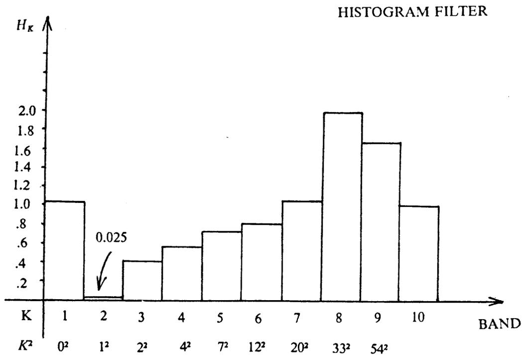
Figure 19. Filter used in histogram method.
