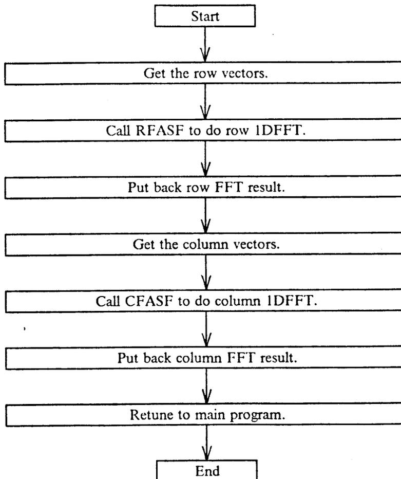
Figure 13. Flowchart for subroutine DIM2FF.
