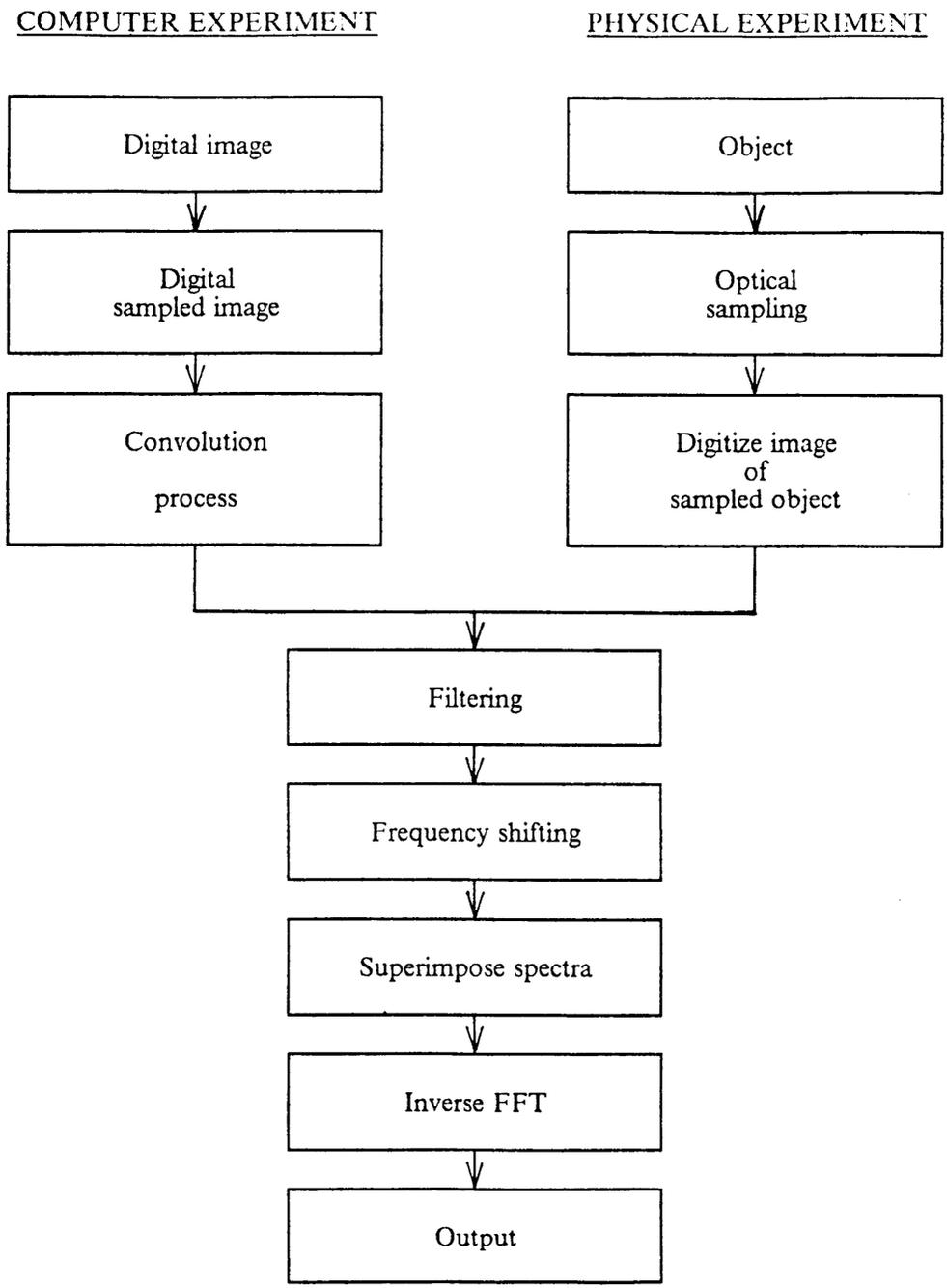
Figure 2. Block diagram of frequency mixing method.
