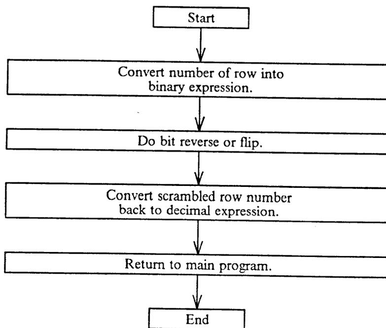
Figure 15. Flowchart for subroutine RSCRBLE.
