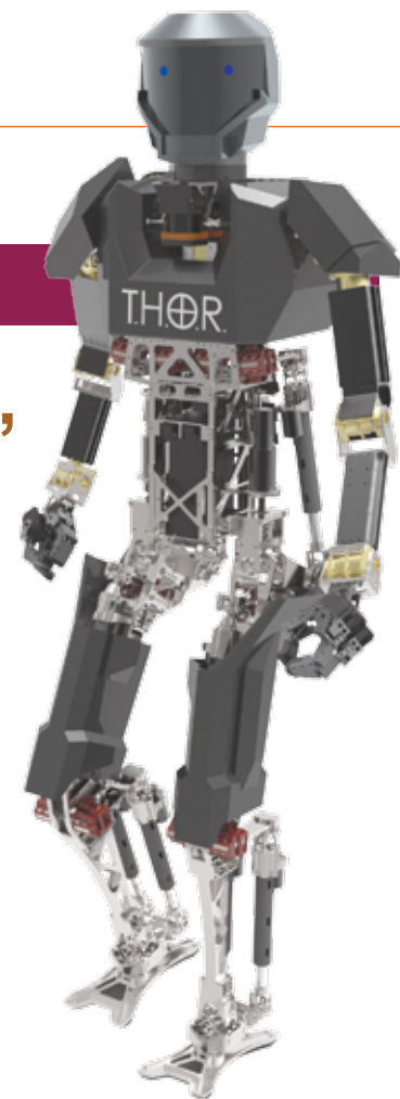
A rendering of Virginia Tech's DARPA Robotics Challenge robot THOR, short for Tactical Hazardous Operations Robot.
