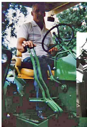
Figure 8. Modified tractor controls for disabled operators: (upper left) tractor controls on the right to accommodate a left-hand amputee; (upper right) spinner knob for steering wheels for better grip and one-hand steering; (lower) hand levers for brake engagement for limited leg mobility or strength.
