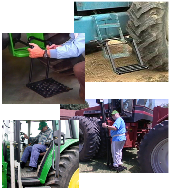
Figure 6. Accessing tractor platform with limited mobility: (upper) extra steps; (lower) platform lifts.
