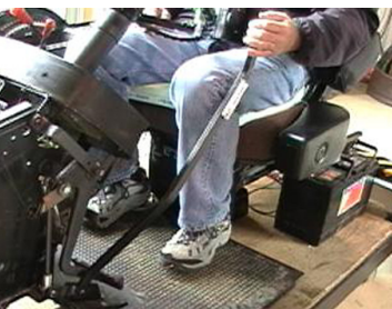
Figure 8. Modified tractor controls for disabled operators: (upper left) tractor controls on the right to accommodate a left-hand amputee; (upper right) spinner knob for steering wheels for better grip and one-hand steering; (lower) hand levers for brake engagement for limited leg mobility or strength.
