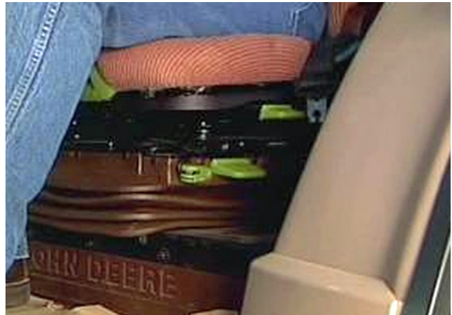
Figure 1. Improved seat suspensions or custom-fitted seats will isolate the operator from low-frequency vibration.
