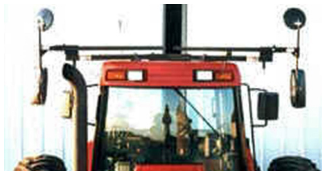
Figure 10. Extra, enlarged, or extended mirrors to reduce neck and back strain.
