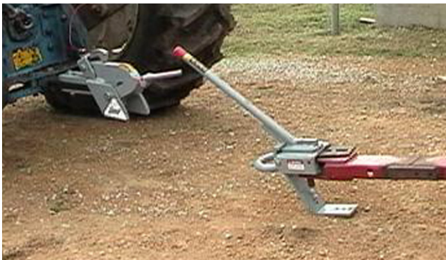
Figure 11. Quick-connect adaptor for attaching implements to drawbar. Farmer remains in the operator's seat and does not dismount for hitching and unhitching the implement.
