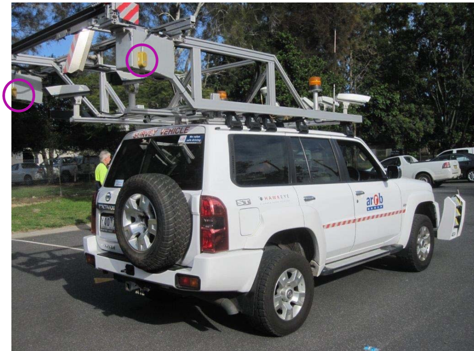
FIGURE 1 3D system with additional accelerometers (circled).
