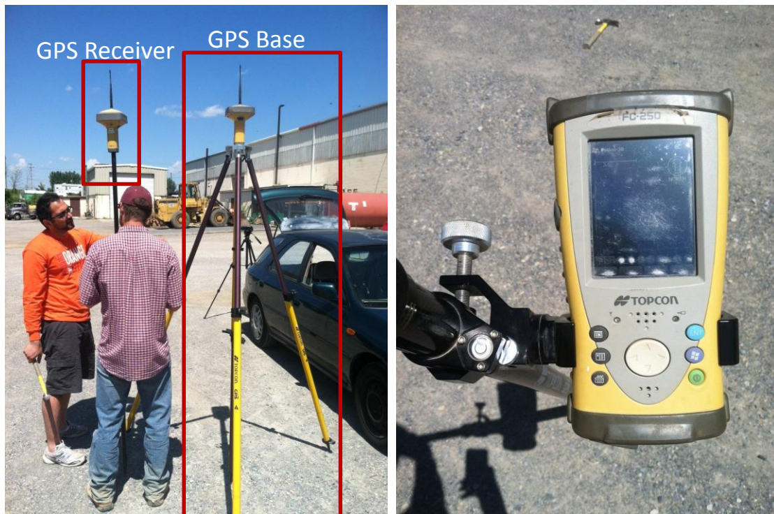
Figure 2.7: GPS unit used to survey the points on the selected paths to benchmark the 3D localization results
