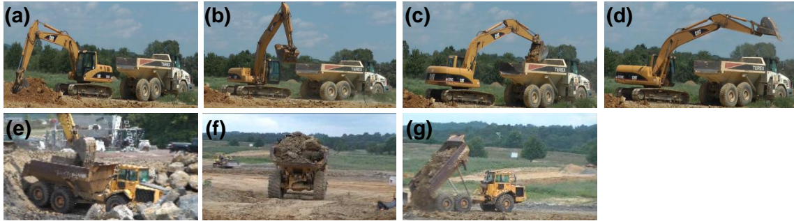
Figure 3.1: Example frames from video sequences in excavator and truck action video datasets: Excavators: (a) digging; (b) hauling (swinging bucket full); (c) dumping; and (d) swinging (bucket empty); Trucks: (e) filling; (f) moving; and (g) dumping.
