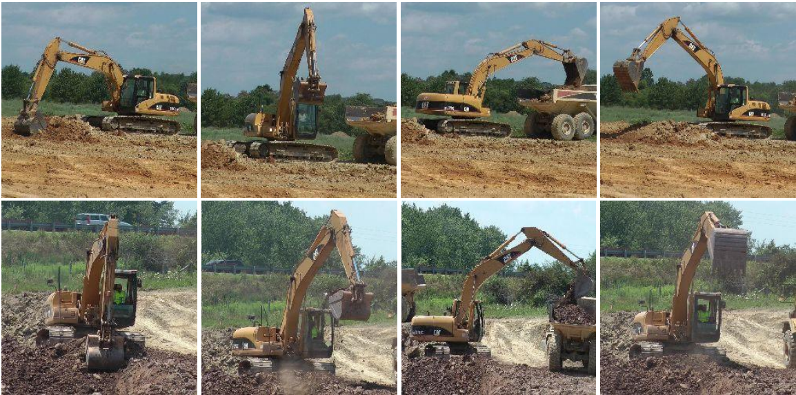
Figure 2.9: Example frames from video sequences of excavator operations. From left to right in rows: digging, hauling, dumping, and swinging action classes which illustrate tremendous appearance changes because of variability in equipment.
