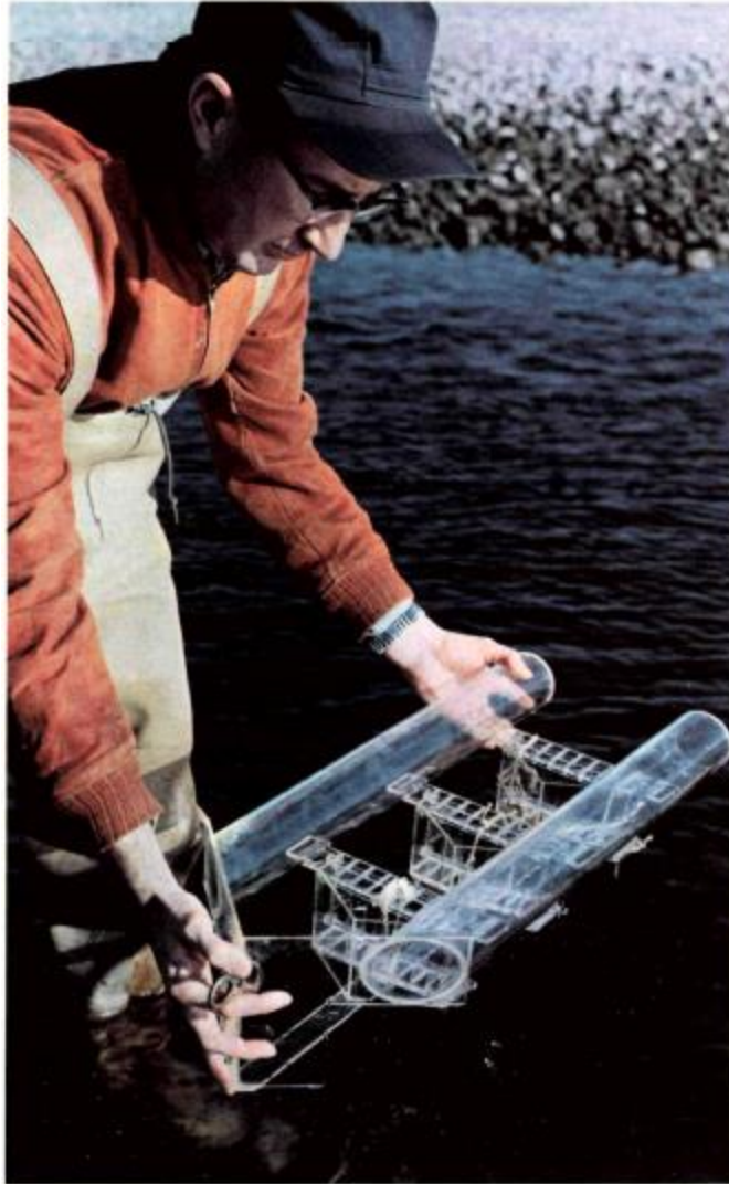
A plankton trap is placed in a river as part of a long-range study of radionuclide uptake by aquatic organisms.
