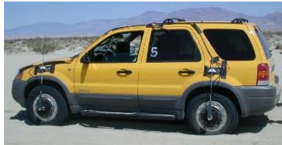
Figure 49. LW12.8 Wheel Load Transducer and its application ( LW12.8, 2017 )
