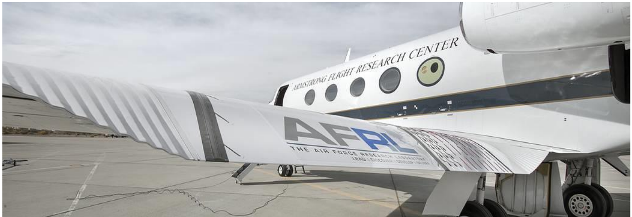
Figure 6 FlexSys and AFRL Adaptive Compliant Trailing Edge [3]
