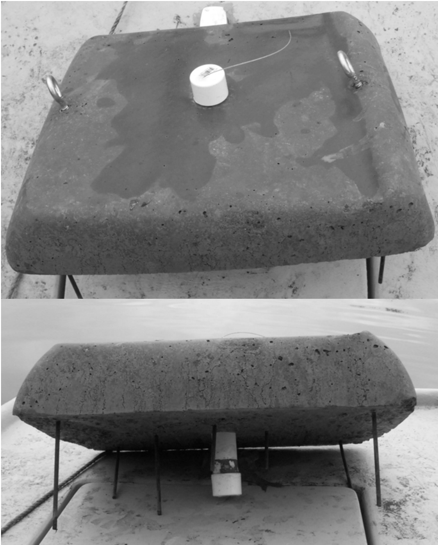
Figure 3.2. Top and side profile of a completed transmitter anchor.
