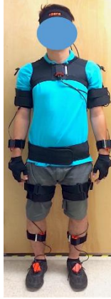
Figure 6-1 The MVN™ system setup using 17 inertial measurement units.
