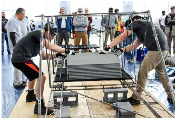
Michael Kokal (left) and Cody Furrow (right) stack 25-pound weights during the vertical load test at the competition. Both needed to work in perfect unison to avoid any mistakes. Credit: Dr. Matthew Hebdon
