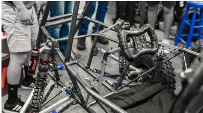
The frame, suspension, and cabin of the Baja car. The car's design includes important mechanical aspects from their previous designs, pictured in the Ware Lab lobby in the photo below.
