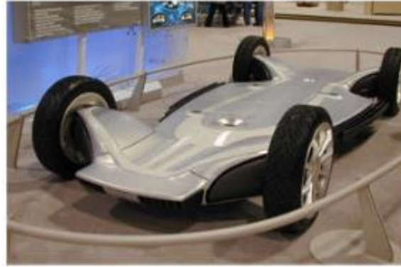
Fig. 1-2. A Skateboard Chassis that contains the electric powertrain, including the ETDS [8].
