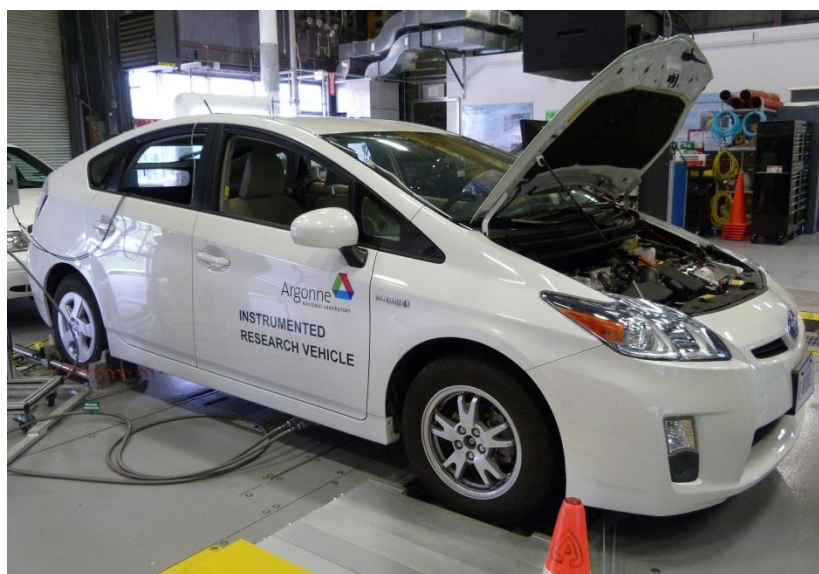
Figure 23. 2010 Toyota Prius test vehicle on the ANL 2WD chassis dynamometer.
