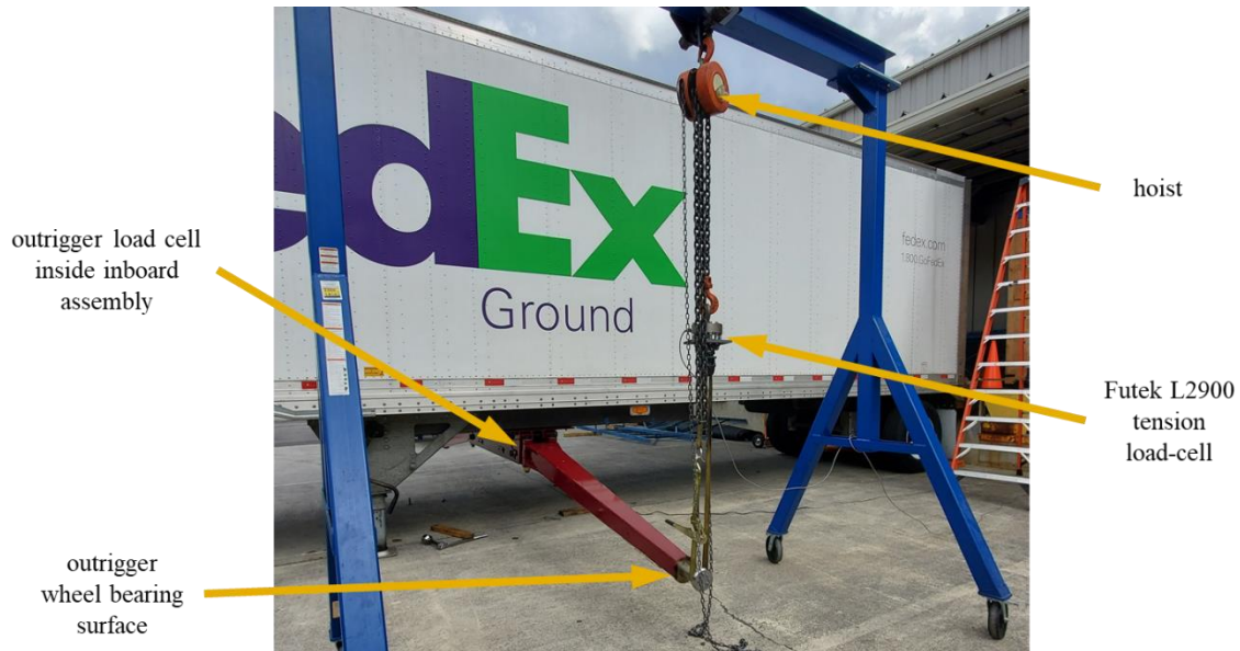
Figure 3-4. Load cell calibration test setup
