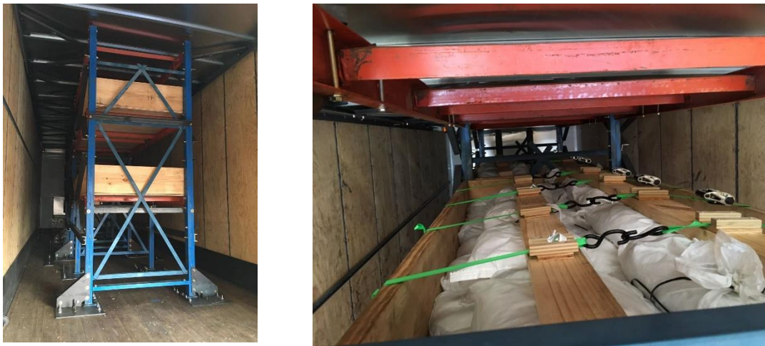
Figure 3-15. Load frame mounted inside the trailers
