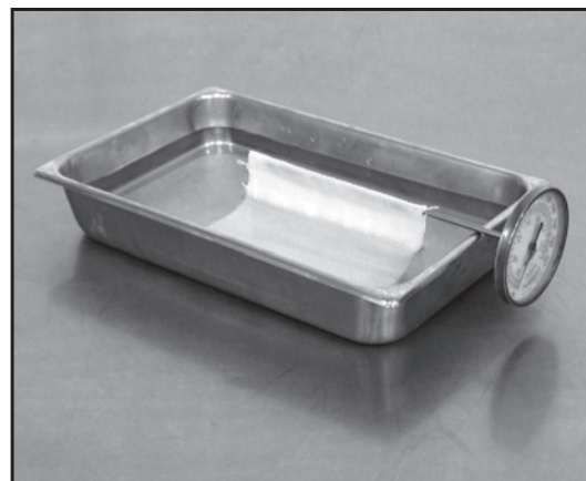
Figures 3a and 3b: Constructing a wet-bulb thermometer.
