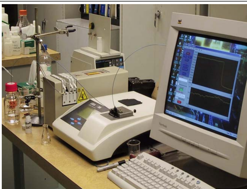
Figure 5.1-1: Leica Microsystems SPR 2001 Alpha System with peristaltic pump (Used with permission of Leica Microsystems Inc.)
