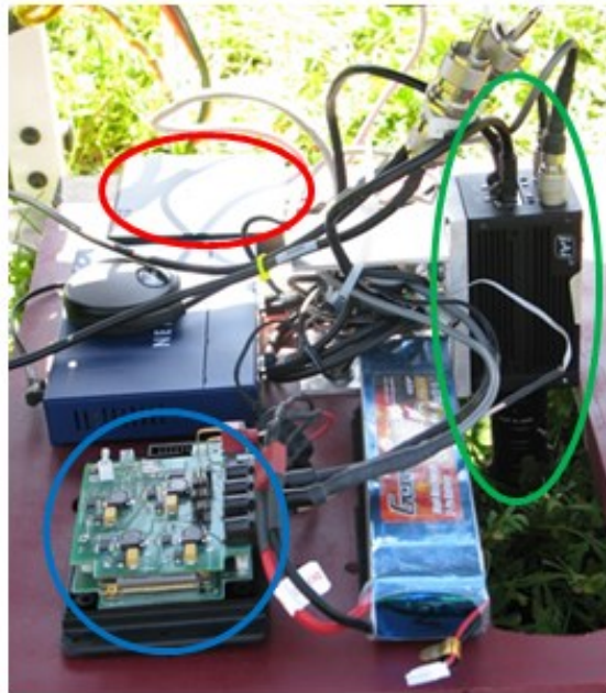
Figure 3.4: The multispectral payload hardware; JAI camera highlighted in green, trigger board highlighted in blue, and fit-PC highlighted in red.
