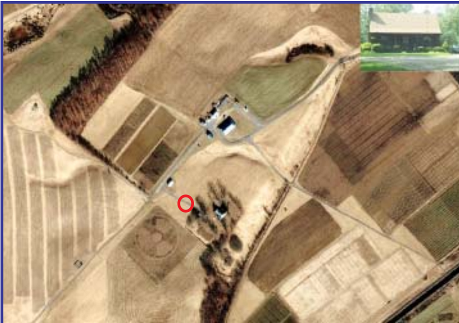
Phase II wireless can associate the geographic location of a cell phone call. Some 911 centers can show the location of the call on an aerial photograph almost instantly.
