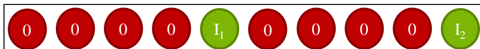
Figure 5-1: An example of a traditional inspection plan, where sampling occurs every 5 products. The products that are sampled for inspection are colored in green and designated with an “I”, whereas the red products are the ones that are not inspected and could be affected by an intelligently designed Product-Oriented C2P attack.
