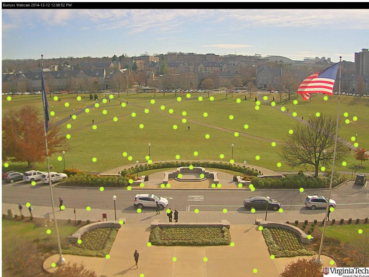
**Figure 2 - Locations on Image where Calibration Points were collected.**
