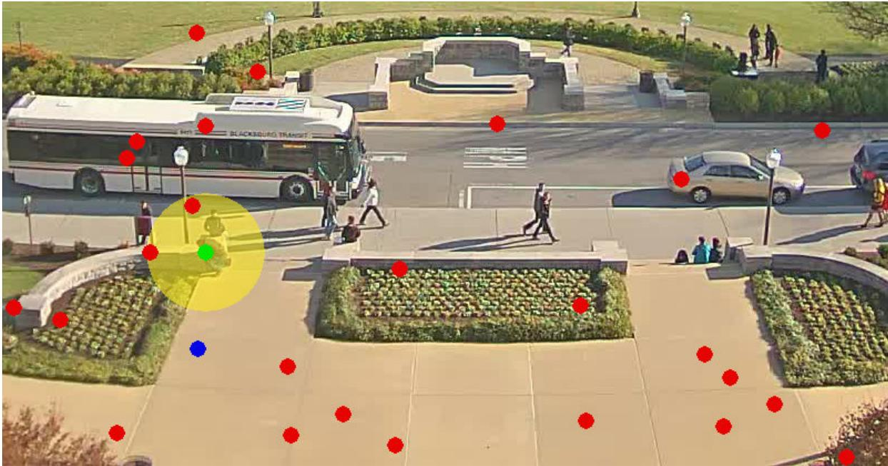
**Figure 8 – Pedestrian Density Test Example.** The iPhone collection point (Green) along with the predicted location (Blue) compared to the 25 Medium-density pedestrian points (Red) randomly generated inside the lower zone. The expected nearest neighbor distance is outlined by the yellow circle.
