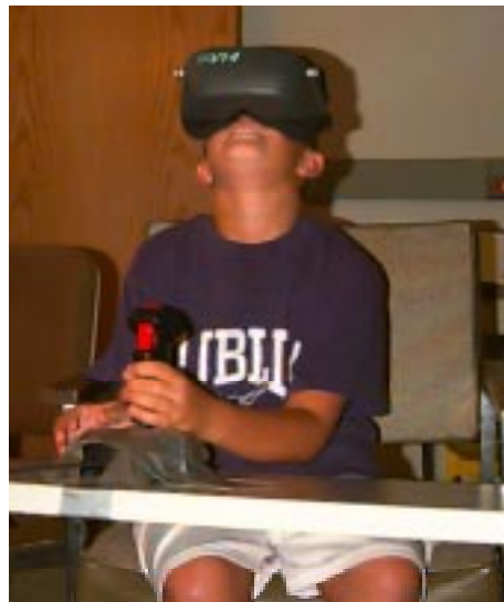
Figure 29. Child tilting head back so that main HMD weight rests on forehead.
