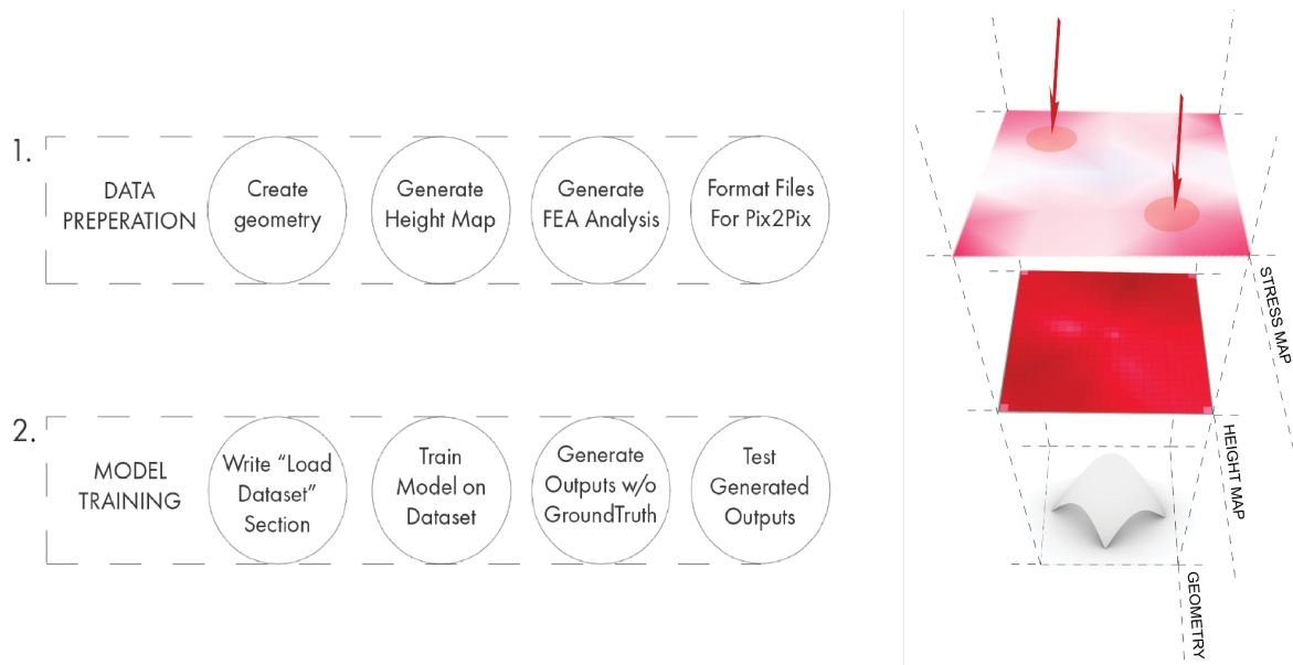
Figure 3: Left: Workflow diagram from creating the dataset to training the cGAN model, Right: Relational diagram of the dataset information
